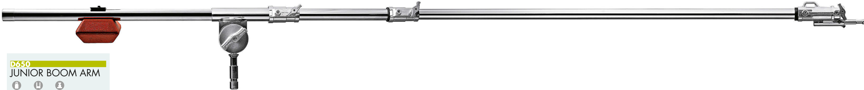
D600 MINI BOOM 3,6kg 7.9lb 16mm 5/8" Min extension 117cm (46.6"). Max load 30kg (66.1lb). Max extension 212cm (83.5"). Max load 7kg (15.4lb). 16mm (5/8") female stand attachment. D600CB MINI BOOM BLACK CHROME FINISH VERSION
